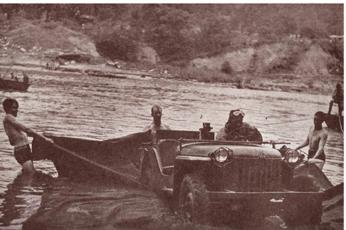
On the cavalry's vehicle list is the bantam jeep which, wrapped in canvas like a canoe, has been floated across rivers by Ft. Riley's Major Charles H. Valentine
